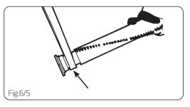
With new belt in place, pull and slide brushbar into nozzle making sure that the brushbar end caps are in the correct orientation (Fig. 6/5 inset). Rotate brushbar manually to make sure belt is properly aligned.
